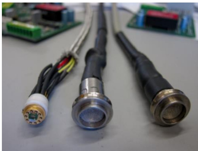
Figure 62. REKO-4: Blank sensor on socket (left), sensor with sintered metal filter cap (center), sensor shrinking hose ready for mounting (right)
