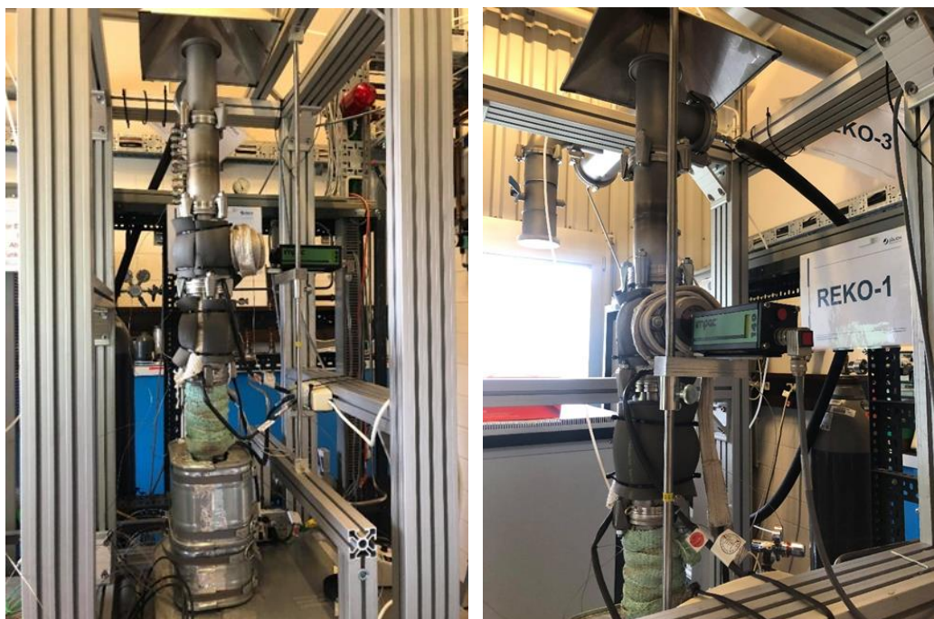
Figure 14. REKO-1: Cylindrical flow reactor (left); catalyst temperature measurement (right)
